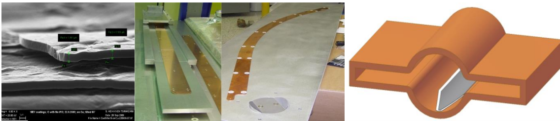
Figure 2.8.2 - Amorphous carbon coating (left) at CERN, clearing electrodes about 1.5 m long before installation in the DAΦNE collider INFN LNF (center) and 3D model of thermal spray tungsten on alumina insulator clearing electrodes (right) for the ILC DR wiggler chambers.
